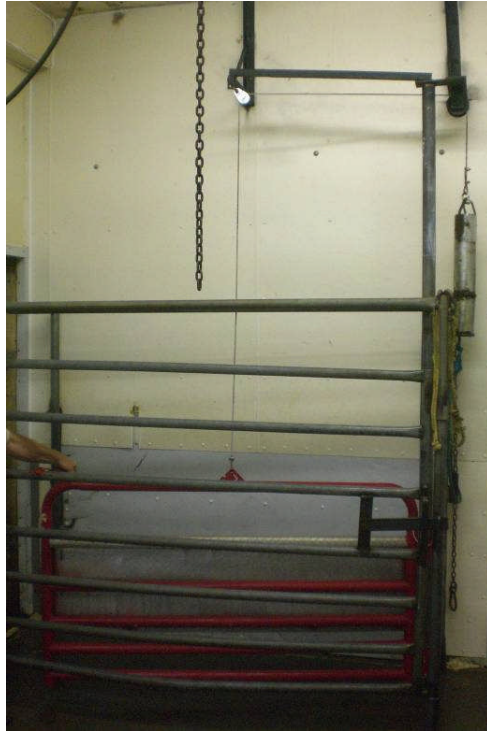
Counter balance weight lowers gate
