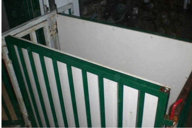
Figure 3: Example of a stun box with plastic “delron” insulation installed.
