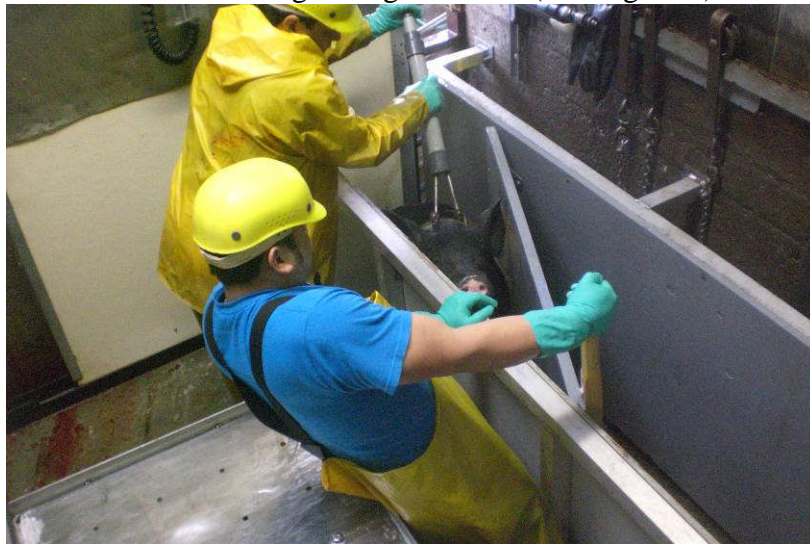
Figure 2: Example of a wood swing gate for restraint during electrical stunning.
