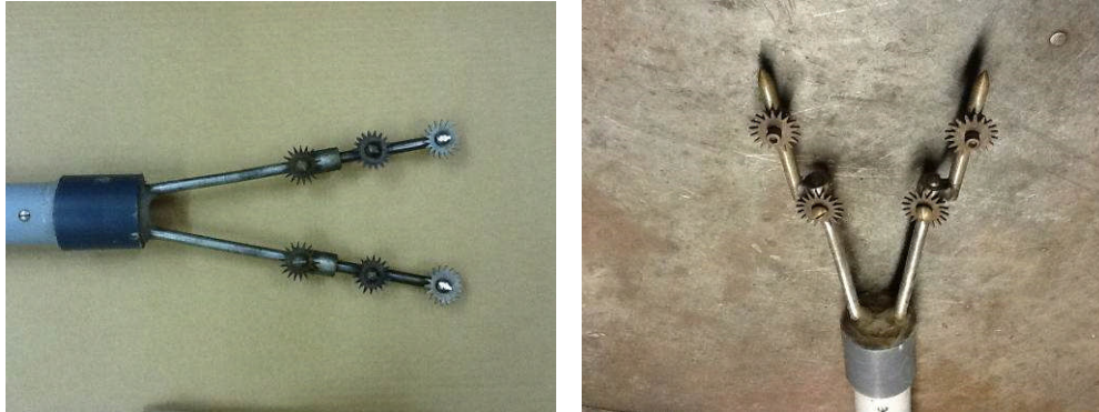
Figure 1: Extend wand length and add star wheels. B&D Extensions added on to wand.
