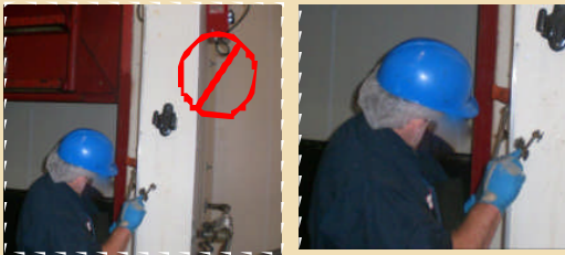
Use a steel brush or a green pad to clean the wand
